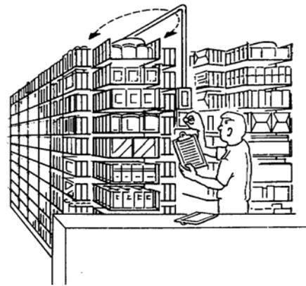
One operator picks from 2 to 4 carousels (termed a "pod") in order to minimize waiting time while other carousels are moving.
