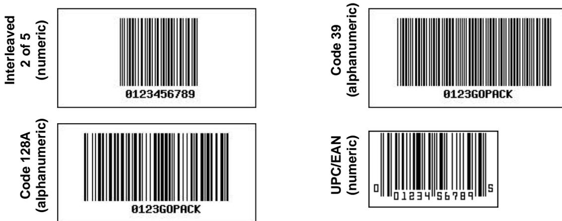
Figure 6.47. Bar codes used in warehousing.<sup>7</sup>
