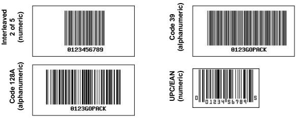
Figure 47. Bar codes used in warehousing.<sup>6</sup>
