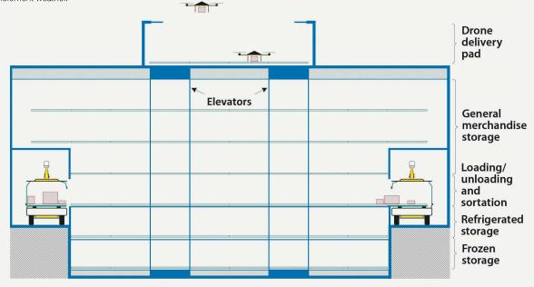
In Figure 3, DDVs are at three of the loading and unloading docks. The DC has seven levels. The top level is for delivery drone loading/unloading, where a retractable roof can close in inclement weather. Three levels below the roof pad provide storage for general merchandise. The next (at grade) level is for loading driverless delivery vehicles, unloading and sortation. And the bottom two (below grade) levels are for goods requiring refrigerated and frozen storage, respectively.
