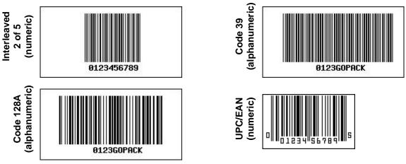
Figure 6.47. Bar codes used in warehousing.<sup>7</sup>
