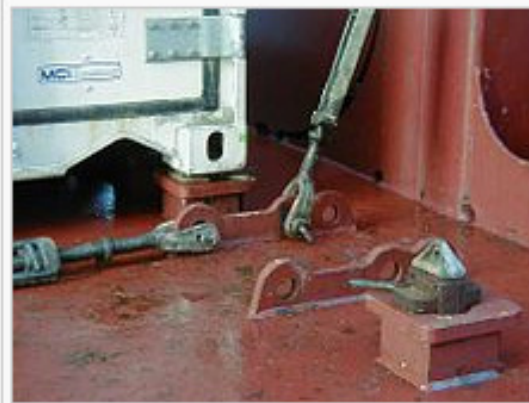
Twistlocks on the base of a container ship. Foreground: unlocked; background: locked. The turnbuckles are "lashing rods" used for additional stability
