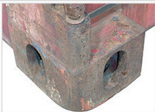
Corner casting on a shipping container . The twistlock proper is done through a larger oval hole on the bottom.
