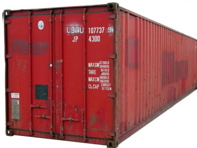
Corner casting on a shipping container . The twistlock proper is done through a larger oval hole on the bottom.
