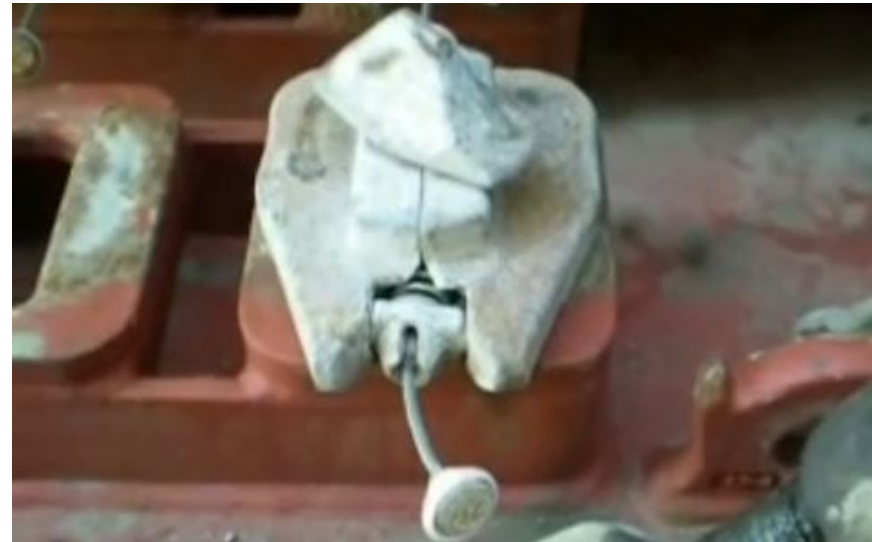
Twistlocks on the base of a container ship. Foreground: unlocked; background: locked. The turnbuckles are "lashing rods" used for additional stability
