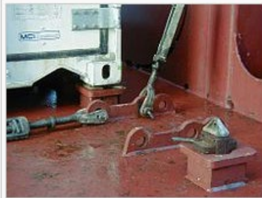
Twistlocks on the base of a container ship. Foreground: unlocked; background: locked. The turnbuckles are "lashing rods" used for additional stability
